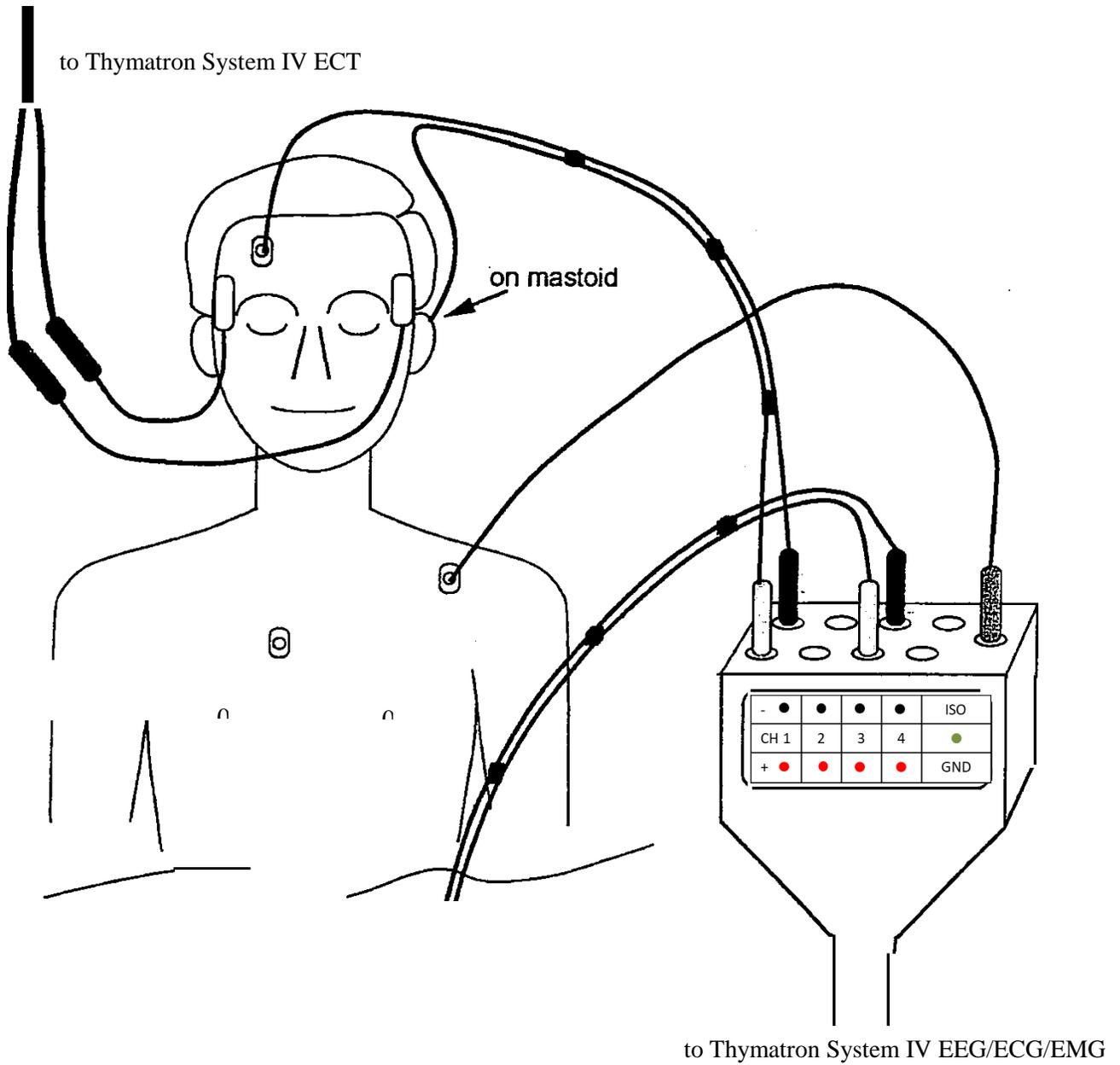
\*Electrode connections for channel 1 EEG, channel 3 EMG recording
