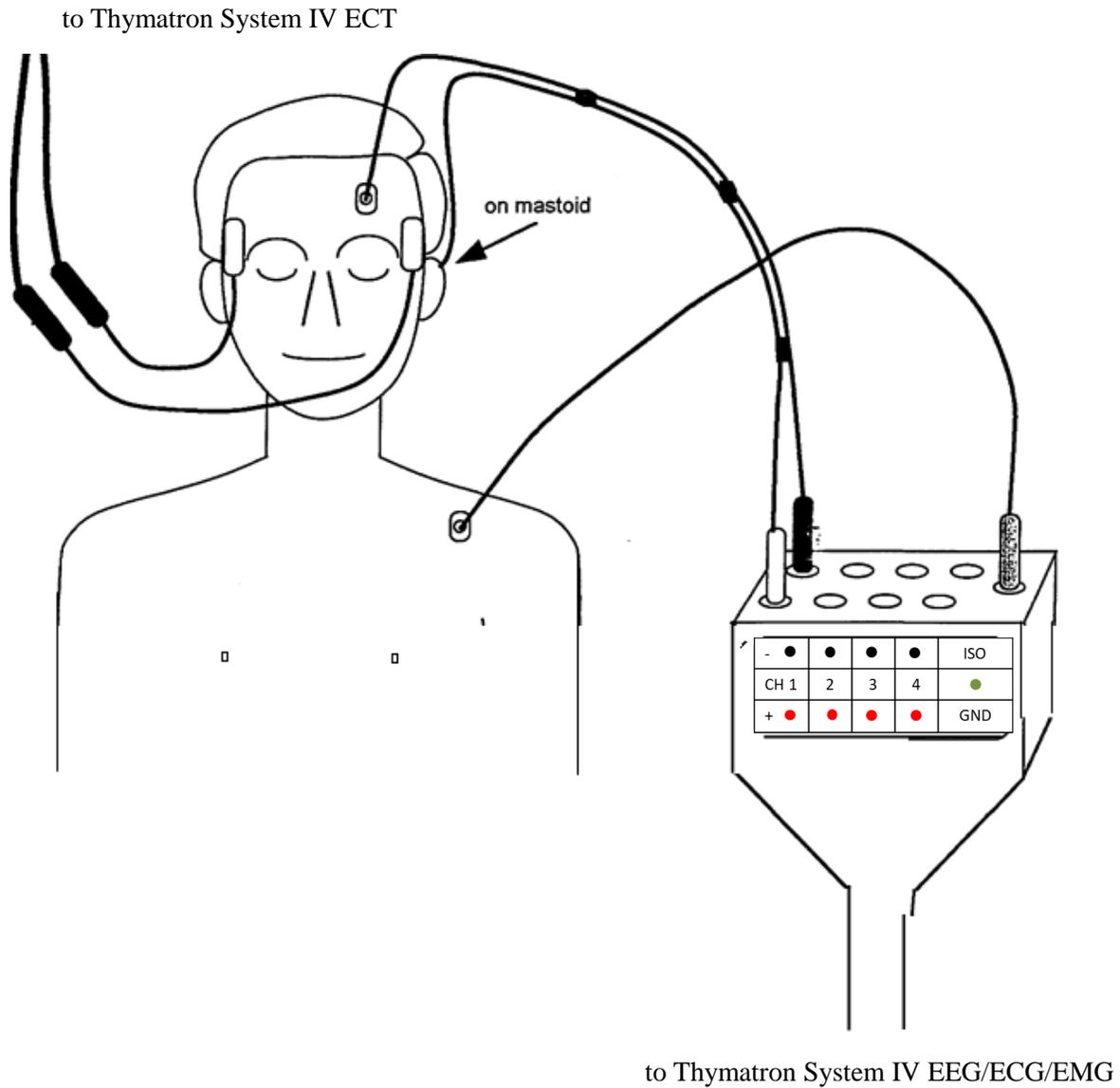
\*Electrode connections for channel 1 EEG recording
